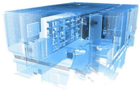
Figure 3. Dense 3D point cloud of an office room for the extraction of single objects.
