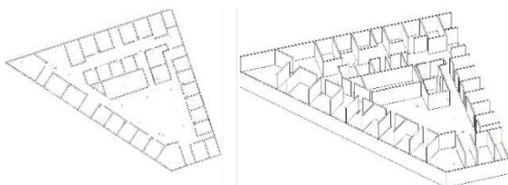
Figure 2. Automatically derived 2D and 3D floor plans from 3D point clouds.
