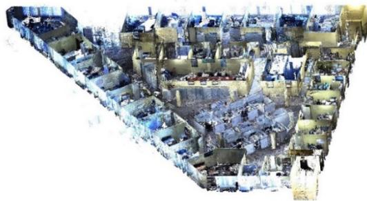
Figure 1. 3D point cloud data captured by a mobile laser scanner (points from the ceiling have been extracted for illustrative purposes).
