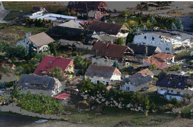
Figure 2. Dense 3D point cloud generated by SfM from images collected by UAV.
