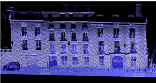
Figure 2. 3D point cloud of building façade.
